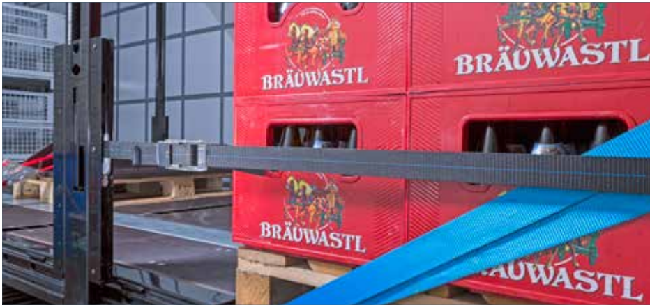
FastFix, the textile lattice by Kögel
