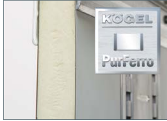
PurFerro sandwich panels: Steel covering layer with PUR foam core, 30 mm thick
